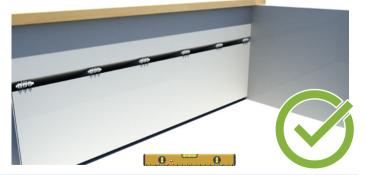
If a deflection is discovered, it can be eliminated as follows: 1] Place a stable wooden beam parallel to the side of the rolloshaft. 2] Remove the middle wheels from the guide rail.
