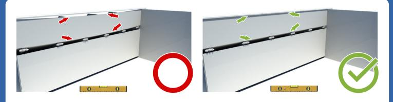
During the backfilling, you must check the flatness of the ceiling and the front side using an aluminum profile. (this is only possible if the wooden frame in this area has been removed)
