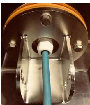
Cable gland screwed into the flange AT-002883
